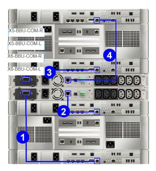
You need to install an XtremlO X1 at a customer's location and want to ensure the correct communication cables are connected to the back of the X- Bricks. Match the cables to their numeric label shown in the exhibit.
