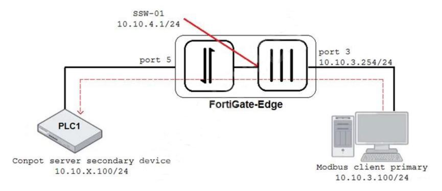
An OT architect has implemented a Modbus TCP with a simulation server Conpot to identify and control the Modus traffic in the OT network. The FortiGate-Edge device is configured with a software switch interface ssw-01.
