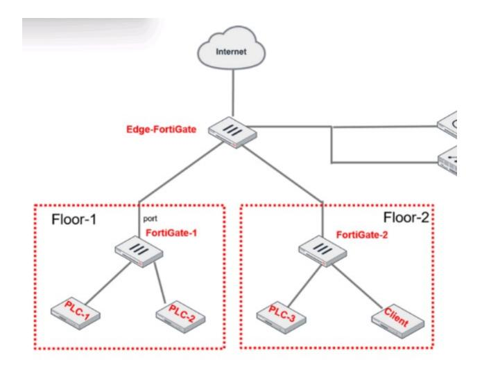
PLC-3 and CLIENT can send traffic to PLC-1 and PLC-2. FGT-2 has only one software switch (SSW-1) connecting both PLC-3 and CLIENT. PLC-3 and CLIENT can send traffic to each other at the Layer 2 level.
