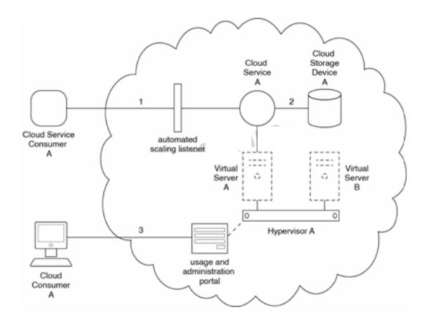
Cloud Service Consumer A accesses Cloud Service A (1), which either sends a query or a read/write request to a database on Cloud Storage Device A (2). A usage and administration portal is available, enabling Cloud Consumer A to view the billing and usage history of Virtual Servers A and B (3).
