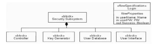
A user provides login credentials to the User Interface, and the Controller passes this information to the User Database The User Database in turn validates the user name and password (typed by PW In the flow Specification) and responds with a Boolean value indicating whether the login was successful. The Controller provides the password to the Key Generator if login was successful.
