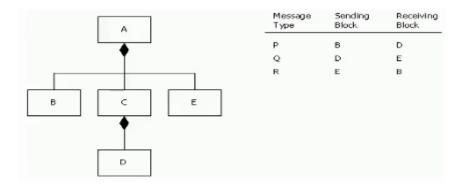
Block C Is encapsulated; none of the other blocks are.
