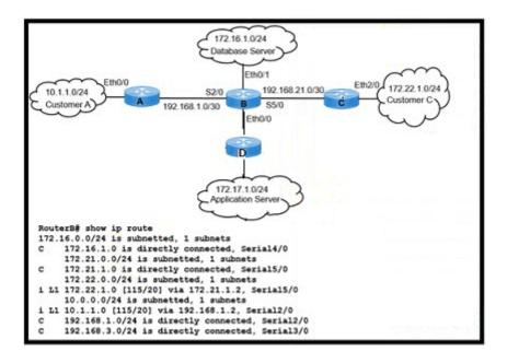
Refer to the exhibit. Customers A and C are experiencing packet drops when connecting to the application server While troubleshooting the problem the network engineer confirms that the IS-IS Level- 1/2 adjacency is up between routers A B C. and D and both customers can communicate with the database server without packet loss Which action must the engineer take to resolve the issue?
