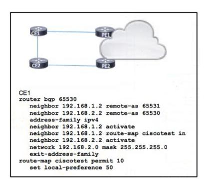
Refer to the exhibit. Routers CE1 and CE2 are in AS 65530. which is multihomed for Internet access. An engineer expects inbound traffic to AS 65530 to arrive from PE1. but it is coming from PE2 instead PE1 and PE2 routers are connected with CE routers through the same bandwidth Which action must be taken to correct the problem?
