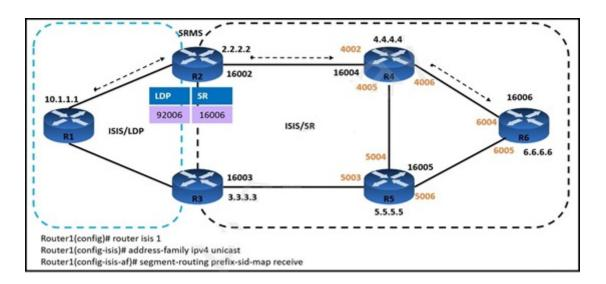
An engineer is configuring service traffic from router R1 to R6 as shown. Which additional configuration must the engineer implement so that the LDP and SR domains will participate and interwork with each other?
