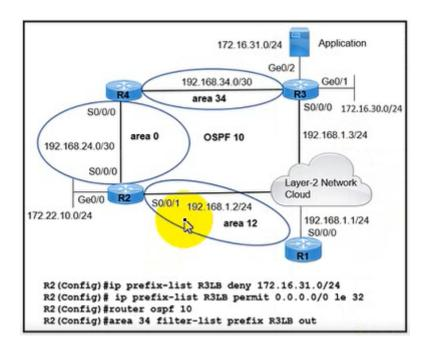
Refer to the exhibit Networks 172.16.31.0/24 and 172 16 30.0/24 are advertised in area 34. and network 172.22 10.0/24 is advertised in area 0. A recent security review discovered that users connected to routers R1 and R2 have been making unauthorized access to an application running on network 172 16 31 0/24 An engineer determined that routers R1 and R2 are receiving updates for network 17 16 31 0/24 Which action resolves the issue?
