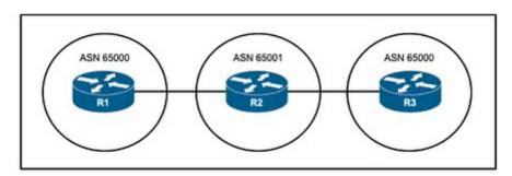
Refer to the exhibit. An engineer is troubleshooting an issue with this network and notices that prefixes from R3 are missing on the R1 routing table Due to repeated ASN when the 10 0 0 0'8 prefix from R3 arrives at R1, BGP automatically rejects it There is no prefix-list on R1 which blocks the traffic from R3 What should the engineer do to fix the problem so that BGP allows that prefix on R1?
