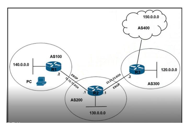
Refer to the exhibit. Excessive routes are flooding from network 150.0.0.0 into AS100. Internet traffic between AS400 and AS300 is working normally. No route controlling mechanism is applied on incoming and outgoing traffic Which configuration resolves the issue?
