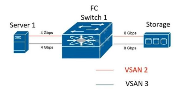
Server 1 fails to connect to the storage array over the Storage Area Network (SAN) of the Cisco NDS 9000 Series Switch. The requirements are to redesign the storage network and keep these considerations in mind:
