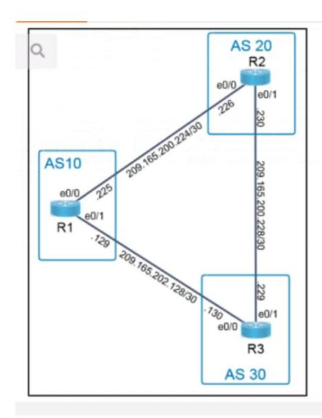
eBGP is configured on R2 and R3. Configure R1 to complete these tasks.
