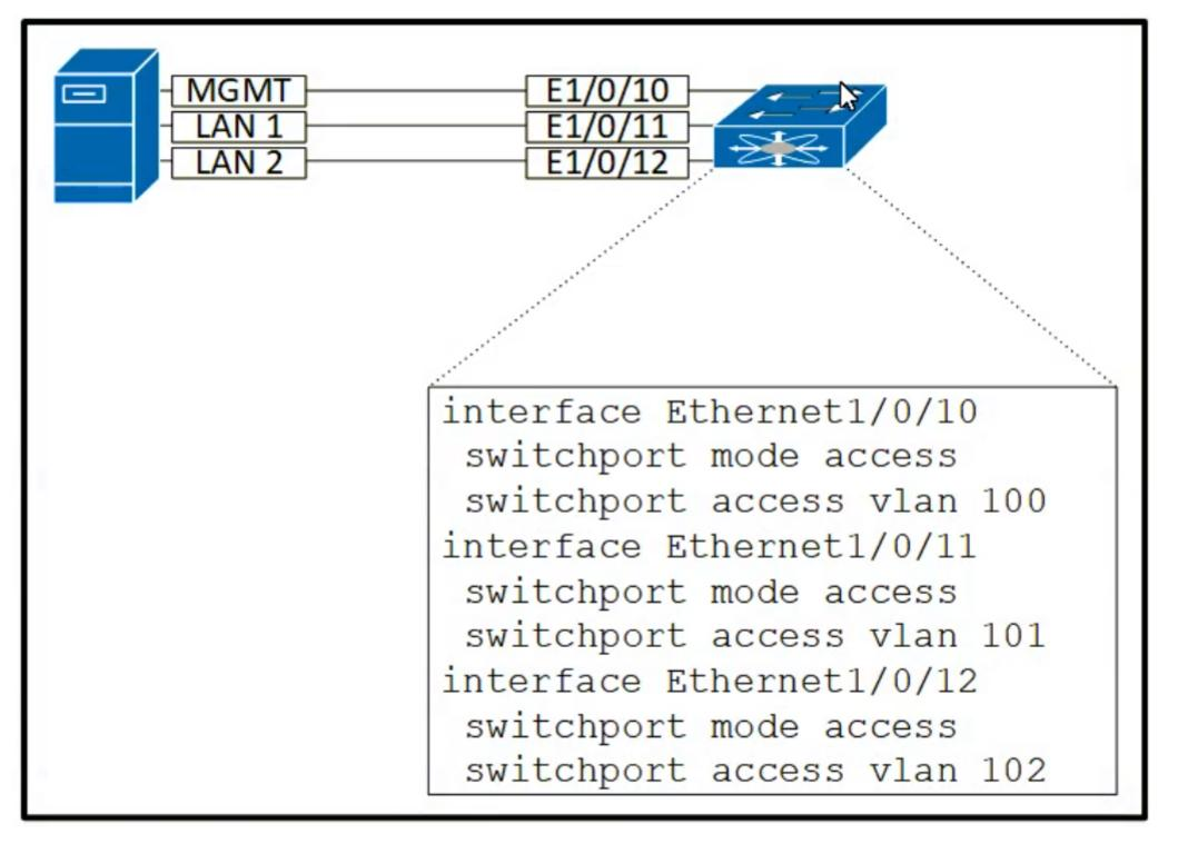
An engineer must access a Cisco UCS C-Series server KVM from a remote location. The engineer must use the out-of-band interface to access the KYM. Which configuration set meets these requirements?
