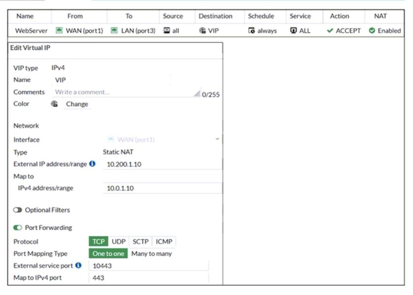
The WAN (port1) interface has the IP address 10.200. 1. 1/24. The LAN (port2) interface has the IP address 10.0. 1.254/24.
