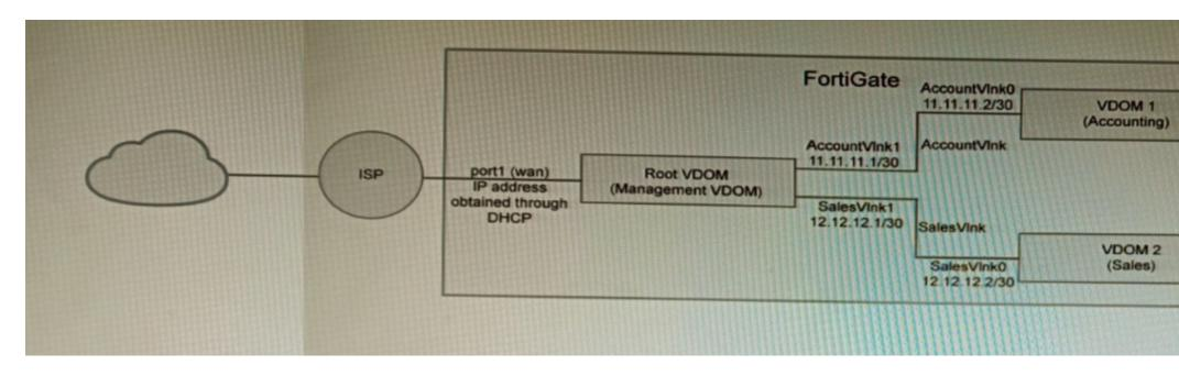
A customer has deployed a FortiGate 300E with virtual domains (VDOMs) enabled in the multi-VDOM mode. There are three VDOMs: Root is for management and internet access, while VDOM 1 and VDOM 2 are used for segregating internal traffic. AccountVInk and SalesVInk are standard VDOM links in Ethernet mode.
