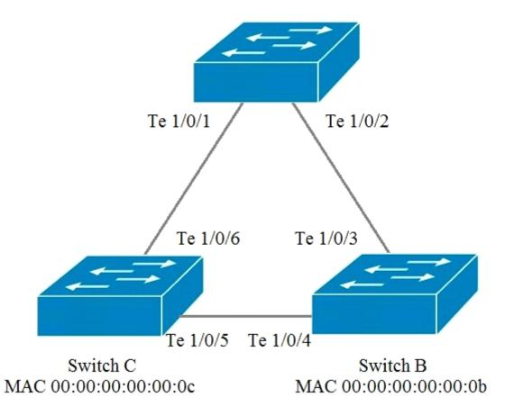
The exhibit represents a topology with all Dell EMC N4000 Series switches with RSTP enabled. In addition, the switches are using the default configuration on all ports and protocols.
