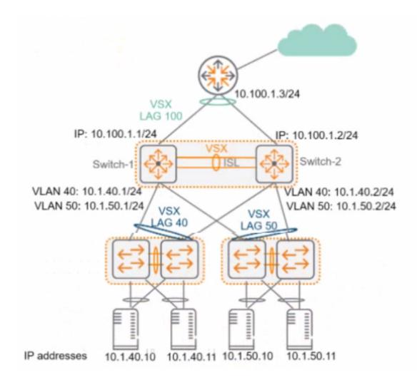
Switch-1, Switch-2, and the router run OSPF on LAG 100, which is a Layer 3 LAG. Does this correctly explain how to control how core-to-access traffic Is forwarded?
