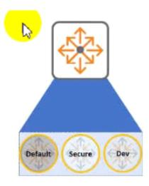
Aruba CX 6300 switch has routes in three different VRFs as per the example above. The user needs to leak routes between VRF Secure and VRF Dev. and also between VRF default and VRF Dev
