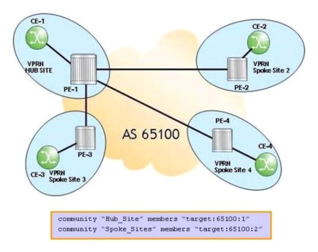
For the PE hub and spoke VPRN, which communities should be imported under the VPRN service on PE2?
