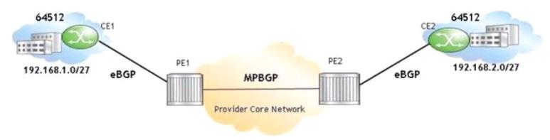
The AS-path nullification method is used to prevent CE2 from discarding routes received from CE1. On which router should the AS-path nullification policy be configured?
