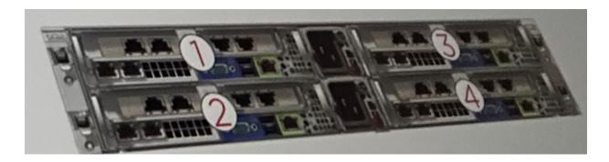
The customer has an existing NX-3160 block and is adding a second node into it.
