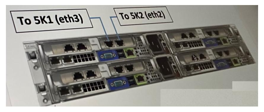
On a four-node NX-3460 cluster, two 10G NiCs are connected to redundant Cisco ToR 5K switches as shown in the first exhibit Port On a four-node NX-3460 cluster, two 10G NICs are connected to redundant Cisco TOR Sk switches as shown in the fist exhibit. Port failover must be tested.
